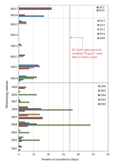
Fig. 8 The number of exceedences over the EU limit value at the individual monitoring stations. It should be noted that the exceedences presented in the figure are those based on the 24 h average limit values using the non-reference instruments for the durations when wind was blowing from construction sites towards the monitoring stations.
