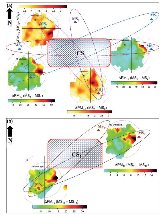
Fig. 4 The polar plots for the paired monitoring stations across each construction site, for  $\Delta PM_{10}$  and  $\Delta PM_{2.5}$  (a) at  $CS_1$  and (b) for  $\Delta PM_{10}$  at  $CS_2$ , respectively. These plots are presented as smoothed surfaces, showing that the concentrations vary depending on the local wind speed and wind direction.
