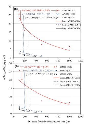
Fig. 9  $\Delta PM_{10}$  and  $\Delta PM_{2.5}$  concentration decay at CS<sub>1</sub> and CS<sub>2</sub> versus the distance in the direction of wind blowing from the construction sites showing the (a) logarithmic and (b) exponential best fit functions. In the fitting equations, x and y express the distance from principal construction site and the PM<sub>10</sub> values, respectively. The solid lines represent the best fitting decay curves.
