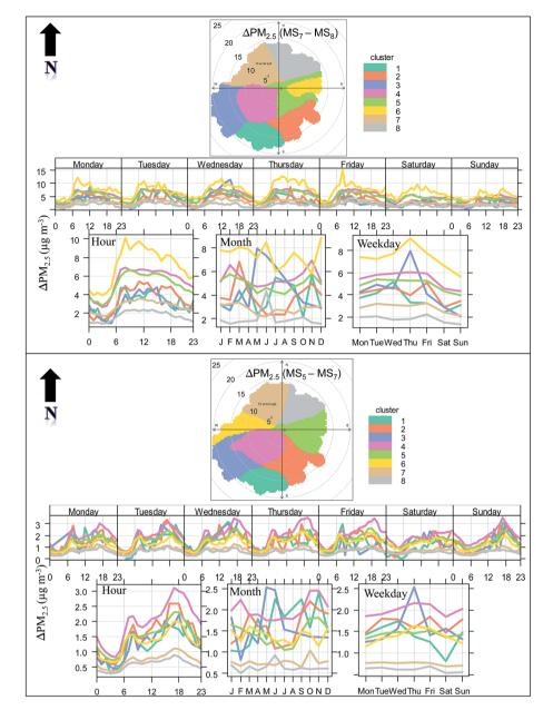
Fig. 6 Clusters identified at CS<sub>1</sub> for PM<sub>2.5</sub> concentrations for 8 clusters. The shading shows the 95% confidence intervals in the mean. The data have been normalised in each case by dividing by the mean.
