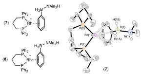
Fig. 3 X-ray molecular structure of (7).  $[BAr^F_4]^-$  anion and selected H atoms omitted for clarity. Ellipsoids shown at 50% probability level. Selected bond lengths (Å) and angles (°): Rh(1)-P(1) 2.2441(11), Rh(1)-P(2) 2.2422(10), Rh(1)-Ph centroid 1.851, B(1)-N(1) 1.618(6); P(1)-Rh(1)-P(2) 94.27(4).
