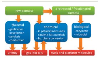
Fig. 3 Schematic representation of the different modes of biomass
