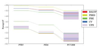
Fig. 3 Calculated (PBE, PBE0, and B3LYP levels of theory) and experimental (cyclic voltammetry/CV and ultraviolet photoelectron spectroscopy/UPS) HOMO and LUMO energy levels for ternary system of PTB7, PID2, and PC71BM.
