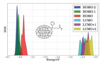
Fig. 5 Density of states (DOS) of calculated B3LYP HOMO-2, HOMO-1, HOMO, LUMO+1, and LUMO+2 energy levels (eV) for 80 PC71BM configurations, with each energy level marked by color. A Gaussian broadening of 0.02 eV was applied to computed energy levels.
