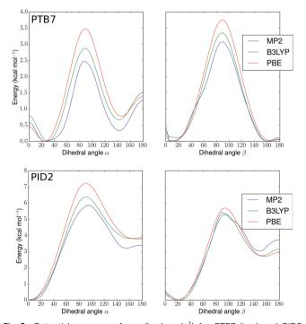
Fig. 2 Potential energy surfaces (kcal mol $^{-1}$ ) for PTB7 (top) and PID2 (bottom) monomers  $versus~\alpha$  and  $\beta$  dihedral angles in degrees (see Fig. 1). MP2, B3LYP, and PBE denote different levels of theory (see text).
