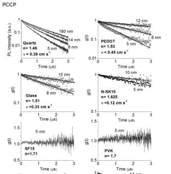
Fig. 6 Ratio of the phosphorescence intensity g(t) measured for neat thin films of IrG1 of given thicknesses to that in the thick film on different substrates, n is the refractive index of the substrate at the PL peak. Solid lines are fits to an exponential decay and surface quenching velocities v obtained using eqn (3) are given.
