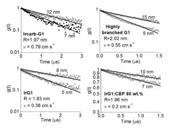
Fig. 3 Ratio of the phosphorescence intensity q(t) measured for thin films of given thicknesses on fused silica substrates to that of the limiting case of a thick film. Solid lines are fits to an exponential decay and the values of the surface quenching velocities v obtained using eqn (3) are given for each material as insets. R is the average intermolecular spacing between the iridium(III) complex cores.
