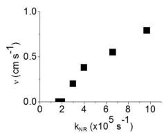
Fig. 5 Surface quenching velocity v in thin films as a function of the non-radiative decay rate  $k_{\rm NR}$  in the bulk films.
