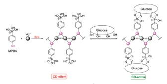
Fig. 9 Interactions of glucose with Ag<sup>+</sup>-MPBA coordination polymers. Reprinted with permission from Chem. Commun., 2015, 51, 8017-8019. Copyright 2015 RSC.
