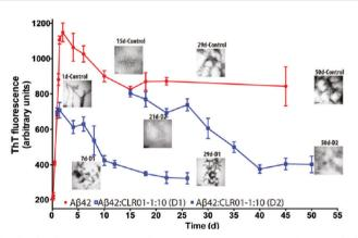
Fig. 5 CLR01 disaggregates Aβ fibrils. Disaggregation of preformed Aβ42 fibrils by CLR01 was studied by adding a 10-fold excess of CLR01 to aggregating solutions of 10  $\mu$ M A $\beta$ 42 at 21 h (disaggregation reaction D1) or 15 days (D2) after initiation of aggregation. The reactions were monitored using ThT fluorescence and TEM. Reprinted with permission from J. Am. Chem. Soc., 2011, 133, 16958-16969. Copyright 2011 American Chemical Society
