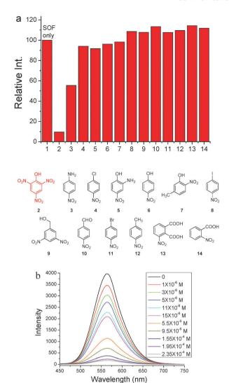
**Fig. 4** (a) Changes in the fluorescence intensity of the 2D SOF upon the addition of different nitroaromatics, and (b) fluorescence spectra of the 2D SOF in the presence of different amounts of PA in water. The concentration of **1** in the SOF was  $2.0 \times 10^{-7}$  M.
