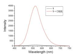
Fig. 3 Fluorescence spectra of **1** (2.0  $\times$  10<sup>-7</sup> M) without and with CB[8] (3.0  $\times$  10<sup>-7</sup> M) in water.  $\lambda_{\text{ev}}$  = 414 nm.
