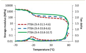
Fig. 2 Dynamic mechanical temperature ramps for solution-cast PTBA films with varying poly(AdA) block length.
