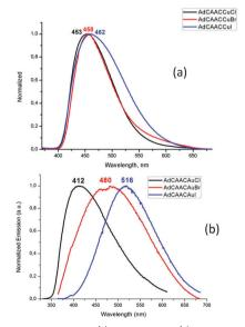
Fig. 2 Emission spectra of (a)  $(^{Ad}L)CuX$  and (b)  $(^{Ad}L)AuX$  (X = Cl, Br, I) in the solid state (excited at  $\lambda_{ex} = 365$  nm).
