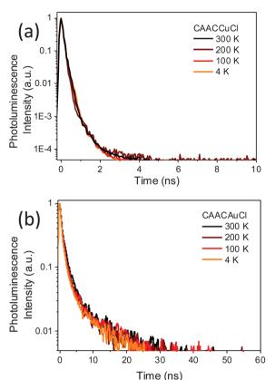
Fig. 3 Normalised PL decay showing singlet prompt decay at different temperatures for (a) 1a, and (b) 2a
