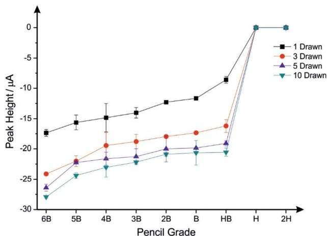
Fig. 3 Plots of pencil composition/grade vs. peak height (cathodic current) recorded in 1 mM hexammineruthenium(III) chloride/0.1 M KCl as a result of increasing the number of draws. Scan rate:  $50 \text{ mV s}^{-1}$  (vs. SCE). Data shown is an average and corresponding standard deviation ( $N = 3$ ).
