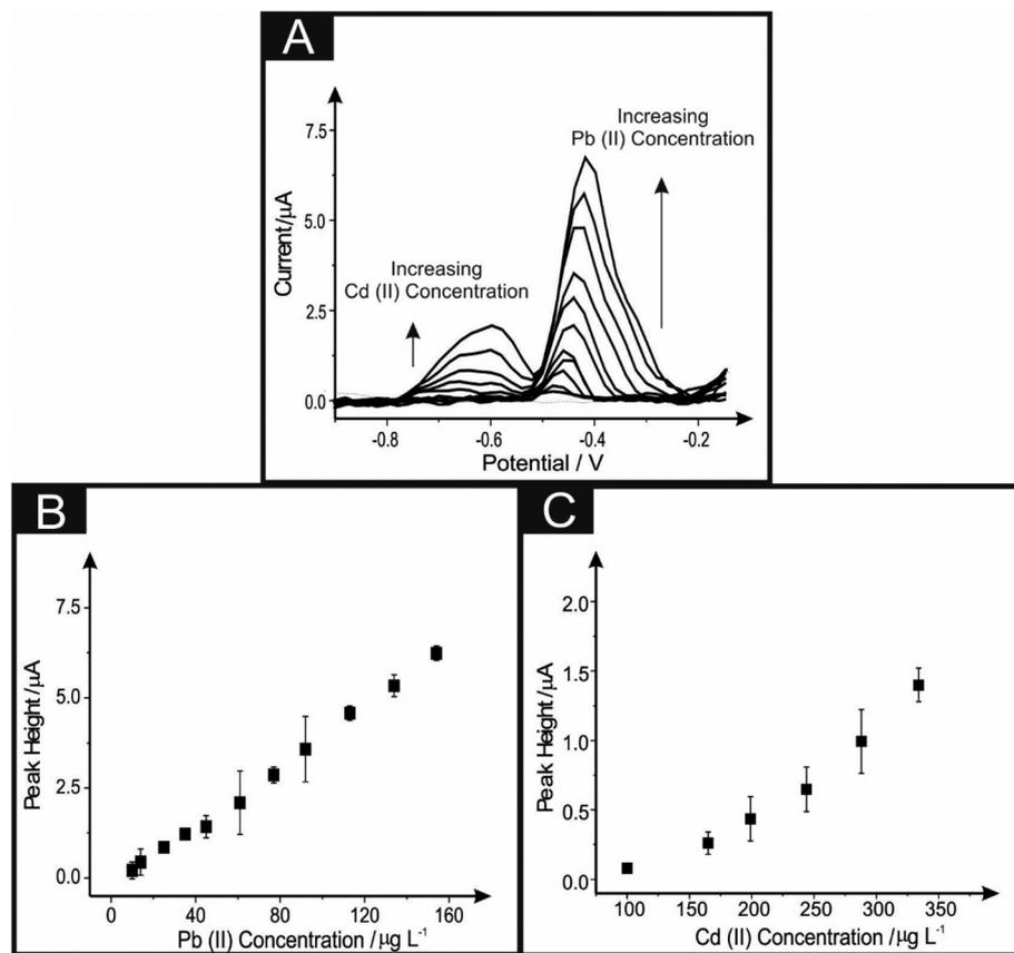
**Fig. 8** Simultaneous determination of Pb(II) and Cd(II) recorded in 0.1 M HCl (dotted line) utilising a back-to-back 6B PDE drawn ten times. Shown in (A) are the corresponding linear sweep voltammograms with corresponding calibration plots (B) and (C) respectively. Error bars indicate the standard deviation of  $N = 3$ . Deposition potential and time:  $-1.2$  V (vs. SCE) and 120 seconds respectively.
