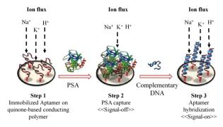
Fig. 7 Working principle for the "off-on" detection of PSA using an aptamer capture probe, followed by hybridization with a complementary sequence (adapted from *Biosens. Bioelectron.*, 2015, 15, 68, 49–54).
