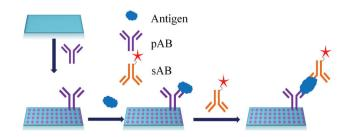
Fig. 16 Detection of PSA on the protein microarray.
