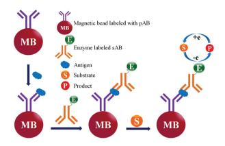
Fig. 6 PSA detection by electrochemical immunoassay.
