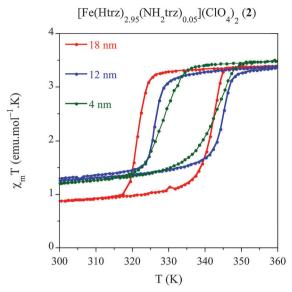
Fig. 5 Temperature dependence of the molar magnetic susceptibility temperature product ( $\chi_M T$ ) for samples **2.1** (18 nm), **2.2** (12 nm) and **2.3** (4 nm) after several heating-cooling modes.
