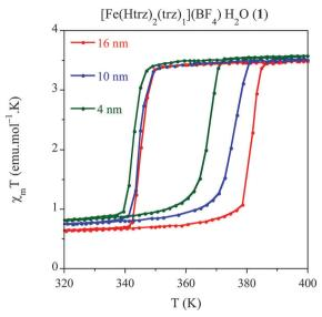
Fig. 4 Temperature dependence of the molar magnetic susceptibility temperature product ( $\chi_M T$ ) for samples **1.6** (16 nm), **1.10** (10 nm) and **1.2** (4 nm) after several heating—cooling modes.
