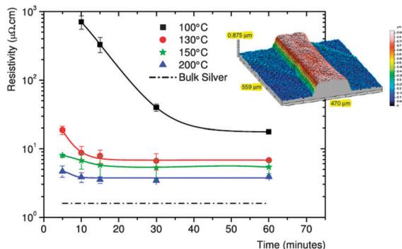
Fig. 12 Electrical resistivity of printed silver lines from a commercial silver ink with 20 wt% of silver as a function of sintering time and temperature reprinted with permission from ref. 115. Copyright (2009) RSC.
