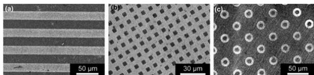
Fig. 7 SEM images of several Ag patterns fabricated by microcontact printing of (3-mercaptopropyl)triethoxysilane (MPTEs) followed by selective electroless plating. (a) Lines with a width of 20  $\mu\text{m}$  and 40  $\mu\text{m}$  pitch, (b) a regular grid with 5  $\mu\text{m}$ -wide lines and (c) rings with an internal diameter of 10  $\mu\text{m}$  and an external diameter of 20  $\mu\text{m}$ . Reprinted with permission from Mondin *et al.*<sup>75</sup> Copyright (2013) Elsevier.
