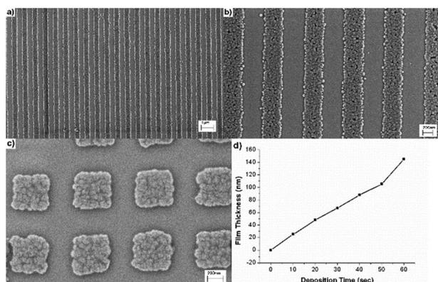
Fig. 8 (a, b) SEM images of Ni lines and (c) SEM image of a pattern of Ni squares, all with a width of 350 nm and a thickness of 60 nm, fabricated by selective passivation from ten Elshof *et al.* (d) Thickness of the Ni structures against deposition time by electroplating. Reprinted with permission from ref. 81. Copyright (2011) American Chemical Society.
