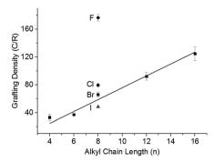
Fig. 4 Grafting density of alkyl halides as a function of alkyl chain length  $(C_nH_{2n+1}Br)$  and halide;  $C_8H_{17}X$  where  $X = F(\spadesuit)$  Cl,  $(\spadesuit)$ , Br  $(\blacksquare)$  or I  $(\blacktriangle)$  for 20 : 1 charged SWCNTs. Line fitted to alkyl bromide series.
