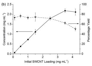
Fig. 3 (a) Influence of C: Na ratio on the concentration of nanotubide solution starting with 3.5 mg mL $^{-1}$  loading of SWCNT. (b) The yield and concentration of nanotubide solutions against initial SWCNT loadings with 20:1 C/Na. Error bars represent standard deviations of 3 repeats.
