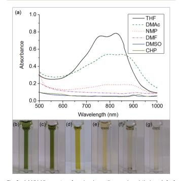
Fig. 2 (a) UV-Vis spectra of equimolar sodium and naphthalene (of  $\sim\!\!1$  mg<sub>(Na)</sub> mL $^{-1}$ ) added to a selection of solvents. (b–g) Cuvettes containing the Na + Np solutions of (b) THF (c) DMAc (d) DMF (e) NMP (f) DMSO (g) CHP.
