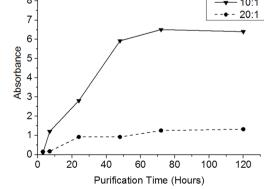
Fig. 6 (a) Concentration of material dissolved *versus* C/Na after 48 h soaking of 1 mg  $\,\mathrm{mL^{-1}}$  SWCNT in DMAc. (b) Absorbance (660 nm) of NaNp/DMAc and SWCNTs at a given SWCNT to sodium ratio *versus* time.
