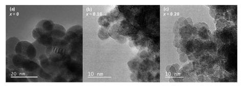
Fig. 3 HR-TEM micrographs of (a) CeO<sub>2</sub>, (b) Ce<sub>0.90</sub>Pd<sub>0.10</sub>O<sub>2- $\delta$ </sub> and (c) Ce<sub>0.80</sub>Pd<sub>0.20</sub>O<sub>2- $\delta$ </sub>.
