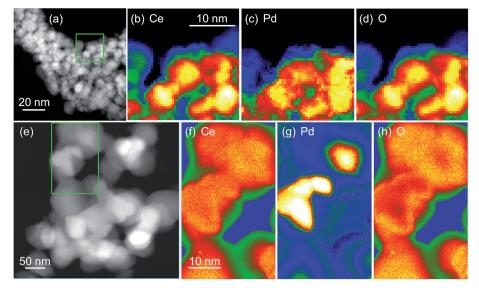
Fig. 7 HAADF images of crystallites in 5 mol% Pd-CeO $_2$  (a) before and (e) after heating oxidation in air at 800 °C and Ce M $_{4,5}$ , Pd M $_{4,5}$  and O K EELS maps (b-d) before and (f-h) after oxidation. The green boxes in (a) and (e) show the areas selected for the EELS maps.
