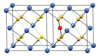
Fig. 1 The CeO<sub>2</sub> structure (two unit cells shown) with one Ce<sup>4+</sup> ion substituted for by a Pd<sup>2+</sup> ion. Pd<sup>2+</sup> is shown in red, Ce<sup>4+</sup> in dark blue and  $O^{2-}$  in orange. The resulting under-coordinated  $O^{2-}$  sites are shown in yellow. This under-coordinated site is 75% occupied to achieve charge-balance.
