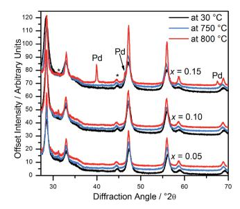
Fig. 5 In situ powder XRD patterns of  $Ce_{1-x}Pd_xO_{2-\delta}$  ( $x=0.05,\,0.10$  and 0.15) at 30 °C, 750 °C and 800 °C. Asterisks denote the position of peaks attributed to the sample holder.
