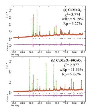
Fig. 3 XRD patterns after final Rietveld refinements for the asprepared products: (a)  $CuMnO_2$  and (b)  $CuMnO_2-40CeO_2$ .
