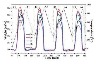
Fig. 8 TGA curves of the as-prepared CuMnO<sub>2</sub>-xCeO<sub>2</sub> samples (i.e., post-annealed at 960 °C for 12 h under flowing Ar) under alternating O<sub>2</sub> and argon. The samples were first oxidized under O<sub>2</sub> to 600 °C, then the gas was switched to argon and the temperature was increased to 900 °C. After being cooled down to 300 °C under argon, the gas was then switched back to O<sub>2</sub> and oxidized to 600 °C.
