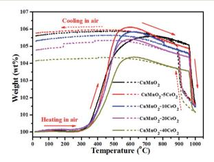
Fig. 6 TGA curves of the as-prepared CuMnO $_2$ -xCeO $_2$  samples (i.e., post-annealed at 960 °C for 12 h under flowing Ar) from room temperature up to 1000 °C with heating and cooling rates of 10 °C min $^{-1}$  under flowing air.
