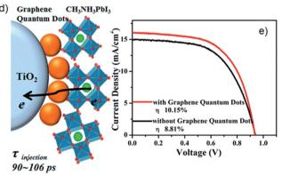
Fig. 8 (a) Schematic of GQD structure. (b) Energy levels of different layers used in PSCs of Zhu et al.,81 (c) Cross sectional SEM image of PSCs fabricated with GQDs. (d) Schematic illustration of electron generation and injection at the interfaces of TiO<sub>2</sub>, GQDs and perovskites. (e) Current density-voltage curves for the best performing PSCs. Reprinted with permission from ref. 81 © 2014, American Chemical Society.
