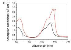
Fig. 2 (a) Absorption of 1 and 2 in chlorobenzene solution (solid lines) and fluorescence excitation spectra (symbols) showing complete transparency in the region of 400 to 425 nm. (b) Absorption spectra of films of 1 and 2 spin coated from chlorobenzene.
