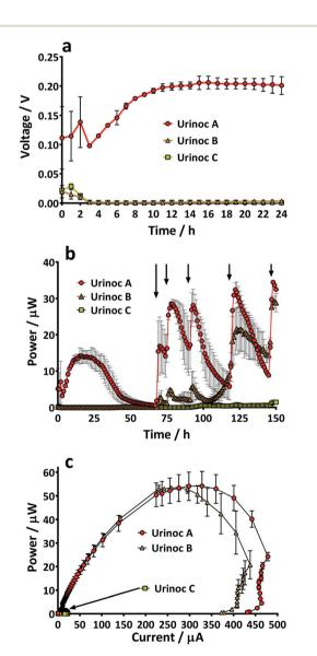
Fig. 5 Comparing different inoculant types in paper MFCs; (a) first 24 hours (under 3 kohm external resistance), (b) actual power produced during first week. Arrows indicate when MFCs were topped up with fresh urine, (c) power curves produced after 2 weeks operation. Data presented as mean (n = 2).
