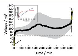
Fig. 7 The recovery of two individual TP-MFCs after 4 weeks refriqeration. MFCs under 950 ohm load. Arrows indicate when MFCs fed fresh urine. Dotted line indicates the voltage required to energise a PMS (not connected). Asterisk indicates when the MFCs were taken down and connected together electrically in parallel. Data presented as mean and range (n = 2), the grey area around curve indicates error bars. Inset shows a magnification of the two individual MFCs during the first 60 min.
