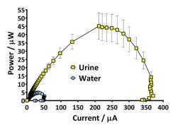
Fig. 10 Power curves generated by TP-MFCs when reactivated with either water or urine. Data presented as mean and range (n = 2).
