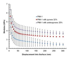
Fig. 8 Comparison of nanoindentation data for unmodified PIM-1 films and PIM-1 films post-modified with either 32% pyrene or 25% 1-aminopyrene.
