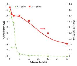
Fig. 4 Gas sorption properties for PIM-1 pyrene blends, nitrogen uptake at 1 bar (obtained from nitrogen isotherms at 77 K) and CO<sub>2</sub> uptake at 1 bar (at 298 K) of PIM-1 and pyrene blends as a function of the composition of the film (trend lines are to guide the eye).
