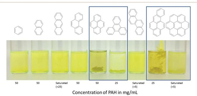
Fig. 3 Effect of the structure of (poly)cyclic aromatic hydrocarbons on the interaction with PIM-1 solution. Three drops of PIM-1 solution (50 ma  $\mathrm{mL}^{-1}$  in DCM) were added to PAH solutions (in at the stated concentration DCM). The cyclic aromatic hydrocarbons and PAHs tested were (from left to right): benzene, naphthalene, anthracene, phenanthrene, pyrene, triphenylene, chrysene, benzo[a]pyrene and coronene. Blue boxes indicate when precipitation was visually observed.
