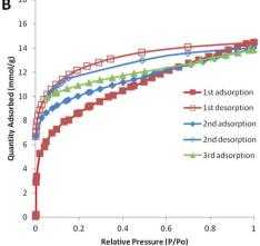
Fig. 5 Cycled adsorption and desorption nitrogen isotherms (77 K). (A) PIM-1 (99%) and pyrene (1%) blend film. (B) PIM-1 film (100%).
