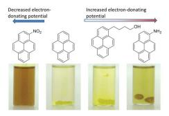
Fig. 6 Effect of addition of changing the electron donating potential of pyrene on the interaction with PIM-1. The image shows the solutions of pyrene derivatives (50 mg  $\rm mL^{-1}$  in DCM) after the addition of three drops of PIM-1 at 50 mg  $\rm mL^{-1}$  (in DCM).
