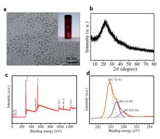
Fig. 1 (a) TEM image, (b) XRD pattern, (c) survey scan of XPS and (d) C 1s core level XPS spectra of the C-dots. The inset in (a) is photograph of C-dots.
