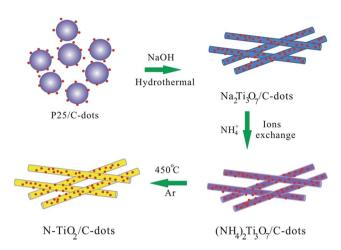
Scheme 1 Illustration for the fabrication process to produce  $N-TiO_2/C$ -dots composite.
