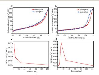
Fig. 5 (a and b) The nitrogen adsorption/desorption isotherm and (c and d) the pore size distribution of (a and c) pure N-TiO<sub>2</sub> and (b and d) N-TiO<sub>2</sub>/C-dots composite samples.
