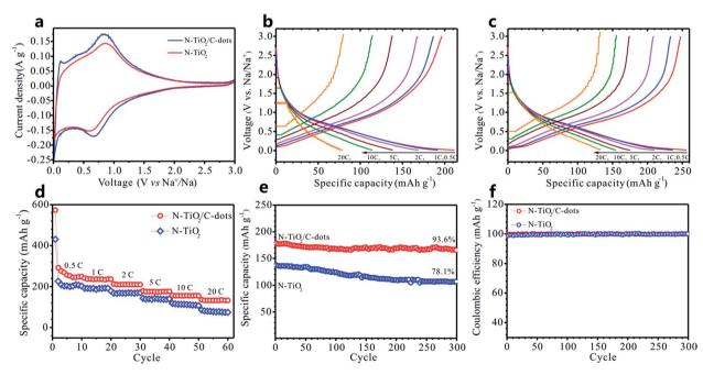
Fig. 7 (a) CV plots of sodium-ion batteries employing the  $N-TiO_2$  and  $N-TiO_2/C$ -dots anodes at a scan rate of 0.2 mV s<sup>-1</sup>. Galvanostatic discharge/charge voltage profiles at different rates of sodium-ion batteries employing the (b) N-TiO<sub>2</sub> and (c) N-TiO<sub>2</sub>/C-dots anodes. (d) Rate capability, (e) cycling performance at 5 C and (f) Coulombic efficiency of sodium-ion batteries employing the N-TiO2 and N-TiO2/C-dots anodes.
