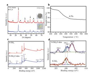
Fig. 4 (a) XRD patterns of N-TiO<sub>2</sub> and N-TiO<sub>2</sub>/C-dots composite. (b) TG analysis of  $N-TiO_2/C$ -dots composite. (c) The survey scan of XPS and (d) N 1s core level XPS spectra of  $N-TiO_2$  and  $N-TiO_2/C$ -dots.
