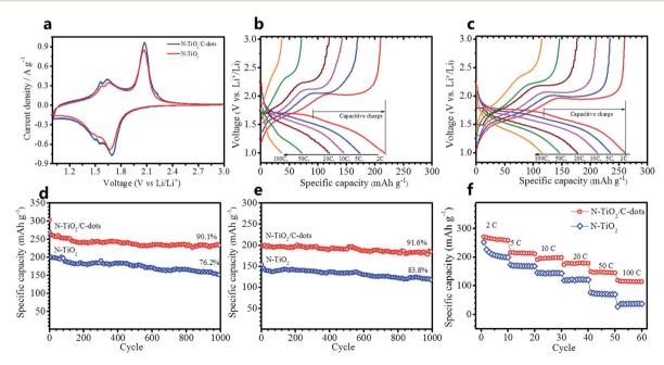
Fig. 6 (a) CV plots of lithium-ion batteries employing the N-TiO<sub>2</sub> and N-TiO<sub>2</sub>/C-dots anodes at a scan rate of 0.5 mV s<sup>-1</sup>. Galvanostatic discharge/charge voltage profiles at different rates of lithium-ion batteries employing the (b) N-TiO<sub>2</sub> and (c) N-TiO<sub>2</sub>/C-dots anodes. Cycling performance at (d) 2 C, at (e) 10 C and (f) rate performance of lithium-ion batteries employing the N-TiO<sub>2</sub> and N-TiO<sub>2</sub>/C-dots anodes.
