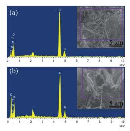
Fig. 3 EDS spectra for the (a) N-TiO<sub>2</sub> and (b) N-TiO<sub>2</sub>/C-dots composite. The insets are the corresponding SEM images.
