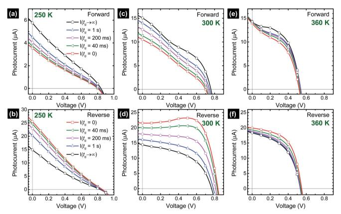
Fig. 5 Photocurrent versus voltage curves composed from the time-dependent data shown in Fig. 2 considering the different delay times (t<sub>d</sub>). The steady-state photocurrent values,  $I(t_d \to \infty)$ , were calculated from the semi-logarithmic plots
