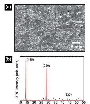
Fig. 1 (a) SEM and (b) XRD characterization of the perovskite film formed from MAI and PbCl<sub>2</sub> precursors.
