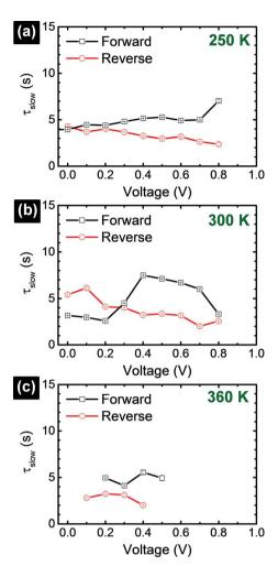
Fig. 4 Extracted time-constants corresponding to the slowest process  $(\tau_{slow})$  observed in the semi-logarithmic plot of the transient part of the photocurrent response upon applied voltage.
