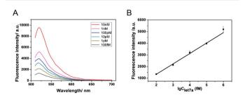
Fig. 3 (A) Fluorescence detection of various concentrations of let-7a (top to bottom: 10 nM, 1 nM, 100 pM, 10 pM, 1 pM, 100 fM). (B) Dependence of the fluorescence intensity at 520 nm on the logarithm of let-7a concentration. The concentrations of Nb.Mva1269I and the MB were 10 units and 200 nM, respectively.
