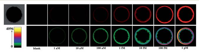
Fig. 2 Microbead brightness as a function of let-7a concentration. Top panel: fluorescence images of the microbeads treated with ascending let-7a concentrations (under PMT HV of 450 V); bottom panel: visualization of the increasing brightness of the corresponding microbeads by using pseudocolor bars where different colors represent different fluorescence intensities.
