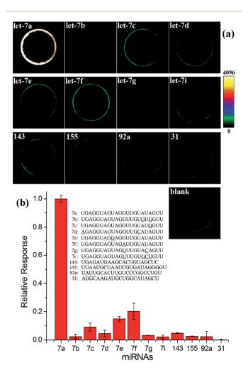
**Fig. 3** Specificity evaluation of the EXPAR-SMBS system. (a) Fluorescence images of the EXPAR-SMBS system with different miRNA targets (PMT HV for the imaging: 550 V); (b) relative responses of other miRNAs compared with that of let-7a. The concentrations of all of these miRNA targets were 10 fM.
