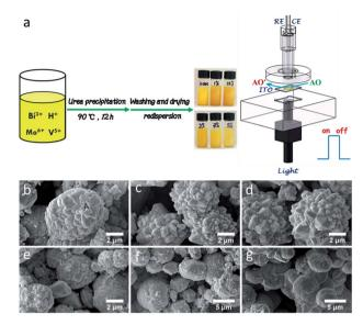
Fig. 1 (a) Schematic illustration for the preparation of  $BiMo_xV_{(1-x)}O_4$  and the PEC process for the AC assay. FESEM images of  $x = (b) \ 0$ , (c) 0.01, (d) 0.015, (e) 0.02, (f) 0.03 and (g) 0.05 for  $BiMo_xV_{(1-x)}O_4$ .
