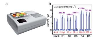
Fig. 6 (a) Photograph of the integrated PEC platform. (b) Photocurrent responses of the  $BiMo_{0.015}V_{0.985}O_4$  modified ITO electrode in the integrated PEC platform without (blank PBS solution) and with the addition of a certain volume of juice to 4 mL of 0.1 mol  $L^{-1}$  PBS (pH = 7.4).
