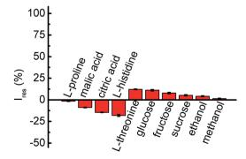
Fig. 5 Photocurrent responses of the BiMo $_{0.015}$ V $_{0.985}$ O $_4$  modified ITO electrode upon the addition of 10 mmol L $^{-1}$  of L-malic acid, 20 mmol L $^{-1}$  of L-citric acid, 25 mmol L $^{-1}$  of L-threonine, 40 mmol L $^{-1}$  of glucose or fructose, 50 mmol L $^{-1}$  of L-histidine, or 250 mmol L $^{-1}$  of L-proline, sucrose, ethanol or methanol in 0.1 mol L $^{-1}$  PBS (pH = 7.4) containing 0.5 mmol L $^{-1}$  GA at 0 V under 470 nm light excitation.
