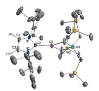
Fig. 2 Molecular structure of 2 with 30% probability displacement ellipsoids. All 3 CH $_2$ SiMe $_3$  groups are disordered. Only one component of the disordered model is shown above. All hydrogen atoms except those on the imidazole ring have been omitted for clarity.
