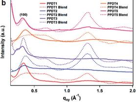
Fig. 5 In plane (a) and out of plane (b) linecuts of polymer (solid lines) and PPDT: PCBM blends (dashed lines). The preferential face-on (100) and (010) polymer peaks are labeled for clarity. The large peak at  $q \approx 1.3$  in the blend films is attributed to PC<sub>71</sub>BM.
