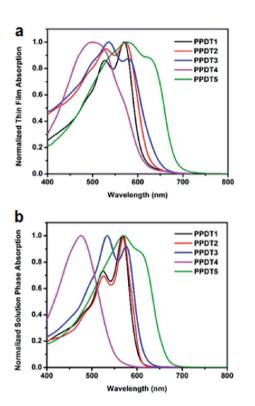
Fig. 2 UV-vis absorption spectra of PPDT polymers. (a) Thin Film Absorption (b) solution phase absorption.
