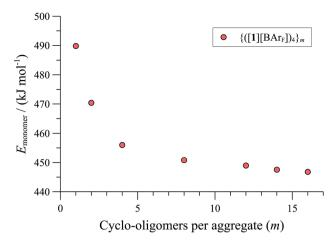
Fig. 7 MM3 energies ( $\varepsilon=9.0$ ) of  $\{([1][BAr_F])_4\}_m$  (normalised per monomer), as a function of number (m) of cyclo-oligomeric tetramers aggregated.
