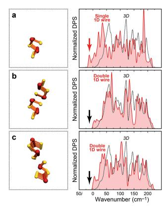
Fig. 6 As Fig. 5, but for single and double 1D "wires" (the supercells employed are much larger than sketched here). The occurrence of imaginary phonon modes in the single wire (a) is emphasised by a red arrow. The double wires in panels (b and c), by stark contrast, are dynamically stable (black arrows). The spillover to marginally "negative" wavenumbers is an artifact of the broadening scheme.
