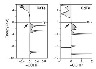
Fig. 4 COHP analysis for the nearest-neighbour contacts in two prototypical telluride materials, *viz.* rocksalt-type CaTe (left) and zincblende-type CdTe (right); structural data from ref. 42 and 43, respectively. The antibonding peak slightly below -8 eV in the CdTe case stems from Cd 4d–Te 5p interactions, as revealed by an orbital-resolved analysis (omitted for brevity). The top of the valence band, however, is devoid of antibonding interactions in both cases (see arrows).
