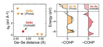
Fig. 8 Bond-projected force constants and COHP analysis for the two GeSe polymorphs (structures and phonon computations for the latter taken from ref. 29;  $\phi_{\rm B}$  and COHP analysis: this work). There are two distinguishable, short Ge–Se contacts in the *Pnma* structure, for which COHPs are drawn with different line styles.
