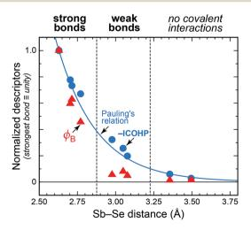
Fig. 7 Bonding descriptors for Sb–Se contacts in crystalline Sb<sub>2</sub>Se<sub>3</sub>. Circles show integrated COHP values at  $\epsilon_{\rm F}$ ; triangles give values of bond-projected force constants (eqn (1)). For comparison, Pauling's measure of bond order (eqn (3)) is shown. All data are given on a normalised scale.
