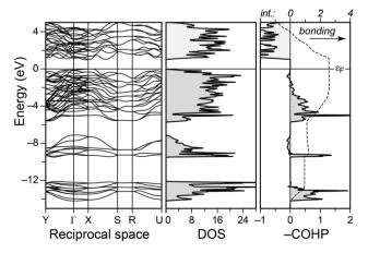
Fig. 2 TB-LMTO-ASA electronic band structure and densities of states (DOS) for Sb<sub>2</sub>Se<sub>3</sub>, and exemplary crystal orbital Hamilton population (COHP) curve for the short Sb(2)–Se(1) contact. The energy integral ("int.") is given by a dashed line. Negative expectation values of the Hamiltonian reflect stabilisation, and thus we plot –COHP as is convention.  $^{30c}$  The Fermi level  $\varepsilon_{\rm F}$  is set as the energy zero.
