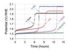
Fig. 7 Accelerated constant current-load durability test (ADT) of Ir-ND OER electrocatalysts in comparison to reference catalysts measured under identical conditions. test time: 15 h,  $N_2$ -purged condition, catalyst loading: 10.2  $\mu q_{lr}$  cm<sup>-2</sup>, 1600 rpm, 10 mA cm<sup>-2</sup>.
