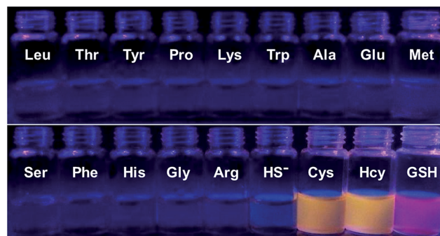
Fig. 3 Fluorescence response of S-S-BODIPY-S in the presence of GSH, Cys, Hcy, \text{HS}^- and other related amino acids. All spectra were acquired at 2.5 h after the addition of the analytes.
