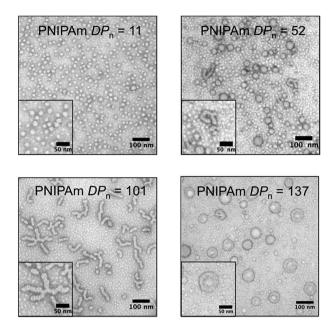
Fig. 4 Transmission electron microscopy of the unpurified crosslinked polymer aggregates showing the progression of nanoparticle morphology as the poly(N-isopropylacrylamide) degree of polymerization (PNIPAm DP<sub>n</sub>) increased (2% uranyl acetate aqueous solution negative stain).
