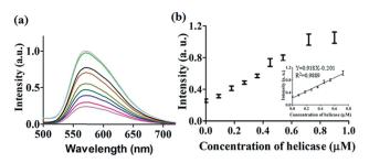
Fig. 3 (a) Luminescence spectra of the 9/G4-quadruplex system in response to increasing concentrations of helicase: 0, 0.09, 0.18, 0.27, 0.36, 0.45, 0.54, 0.72, and 0.9  $\mu\text{M}$ . (b) The relationship between luminescence intensity at  $\lambda=571$  nm and helicase concentration. Inset: linear plot of the change in luminescence intensity at  $\lambda=571$  nm vs. helicase concentration.
