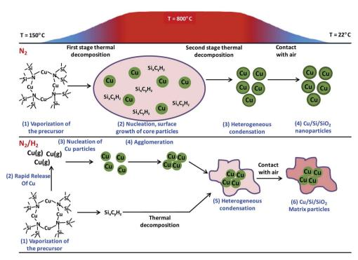
Fig. 11 Schematic representation of formation of Cu-Si/SiO<sub>2</sub> NPs by APCVS process. Reproduced with permission from ref. 233.
