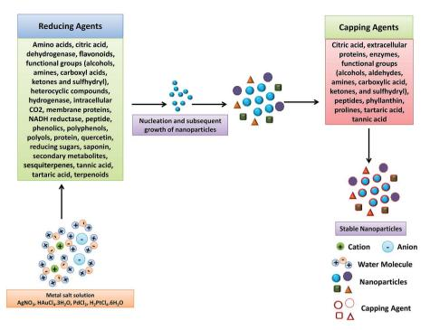
Fig. 15 Mechanism for the biogenic synthesis of metal NPs using plant extract. Reproduced with permission from ref. 305.
