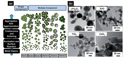
Fig. 8 (a) Formation of different particle configurations via the gas-to-particle mechanism for single and multicomponent systems, (b) asprepared metal oxides NPs of different morphologies made by FSP, varying from hexagonal/octagonal platelet g-Fe<sub>2</sub>O<sub>3</sub>, lightly oblongated ZnO, spherical TiO<sub>2</sub>, and rhomboid-shaped CeO<sub>2</sub> with sharp edges. Reproduced with permission from ref. 118.
