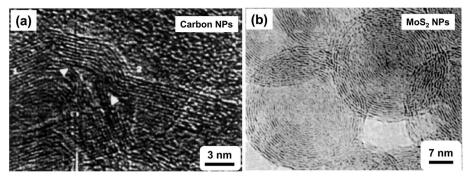
Fig. 6 (a) High resolution electron microscopic image of thin film of carbon cross-linked NPs and (b) high resolution transmission electron microscopic image of thin film of fullerene-like MoS<sub>2</sub> NPs. Reproduced with permission from ref. 108 and 109.
