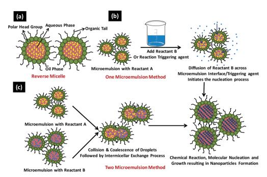
Fig. 9 Shows (a) typical reverse micelle system, (b) various steps involved in one microemulsion process and (c) reaction sequence involved in the two microemulsion nanoparticles synthesis.
