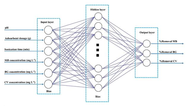
Fig. 2 Schematic of the ANN structure and the basic principles of ANN.
