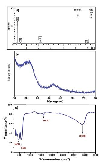
Fig. 5 (a) EDX analysis, (b) XRD pattern and (c) FTIR spectrum of  $MnO_2$ -NP-AC.
