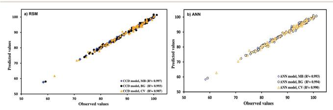
Fig. 6 Predicted vs. experimental data for dyes using (a) RSM and (b) ANN.
