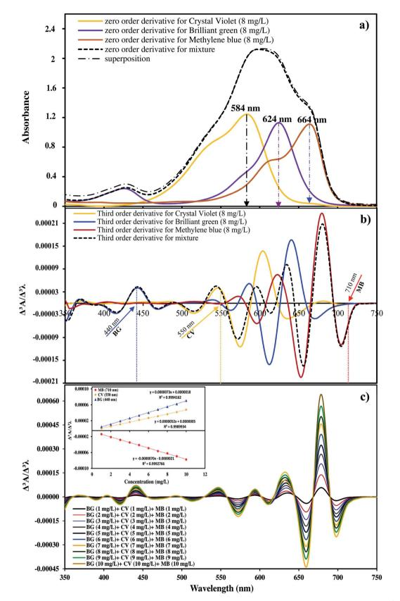
Fig. 3 (a) Zero order absorption spectra of CV, BG and MB in single and ternary solutions (with an initial dye concentration of 8 mg  $L^{-1}$  for each dye). (b) Third order derivative spectra of CV, MG and MB in ternary solutions. (c) Calibration graph at 710 nm for MB, 550 nm for CV and 440 nm for BG.
