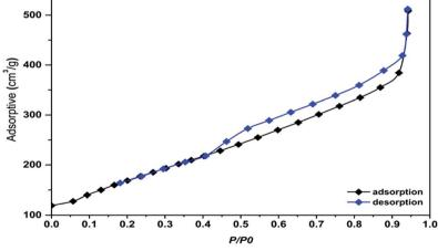
Fig. 4 (a) FESEM image of the prepared  $MnO_2$ -NP-AC, (b) pHzpc of  $MnO_2$ -NP-AC (pH $_i$  = initial pH and pH $_f$  = final pH) and (c) nitrogen adsorption-desorption isotherms.
