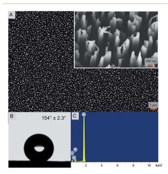
Fig. 1 (A) Electron micrograph of the nanostructured silicon super surface fabricated using DRIE. The inset presents the tilted view of the nanopillars. (B) The super surface displayed a static water contact angle of 154° indicating superhydrophobicity. (C) The EDX spectra of the fabricated silicon showing the presence of elements.
