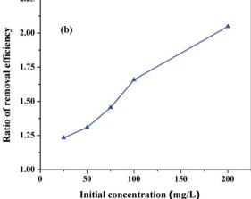
Fig. 7 The comparison (a) and the ratio (b) of Cr(vi) removal efficiency between the modified and pristine biochar.
