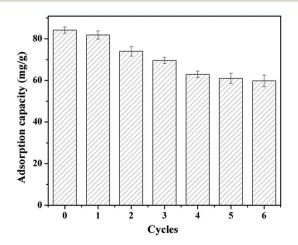
Fig. 13 Sixth consecutive adsorption-desorption cycles of zincbiochar for Cr(vi) removal (volume: 50 mL; adsorbent dose: 0.1 g; initial  $Cr(v_1)$  concentration: 500 mg  $L^{-1}$ ; pH: 2.0; contact time: 24 h).
