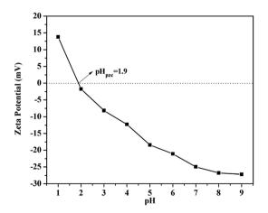
Fig. 6 Zeta potentials of zinc-biochar at different solution pH.
