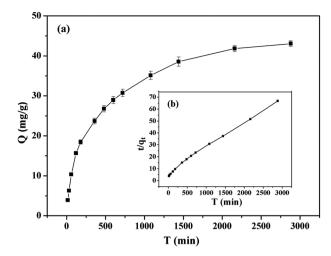
Fig. 9 Kinetics of  $Cr(v_1)$  adsorption onto the zinc-biochar at 303.15 K (initial  $Cr(v_1)$  concentration 100 mg  $L^{-1}$ ; pH: 2.0). (a)  $Cr(v_1)$  sorption kinetics data; (b) pseudo-second-order model for  $Cr(v_1)$  adsorption.
