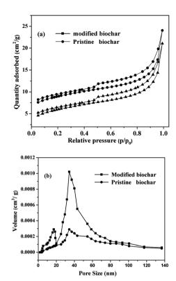
Fig. 4 Nitrogen adsorption—desorption isotherms (a) and pore size distribution (b) of pristine and modified biochar.
