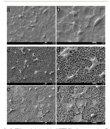
Fig. 7 SEM morphologies of the MC3T3-E1 cells grown on bare Ti substrate (a), HAP coating (c) and ZnCuHAP coating (e); The higher magnification images of the surface of the MC3T3-E1 cells grown on bare Ti substrate (b), HAP coating (d) and ZnCuHAP coating (f).
