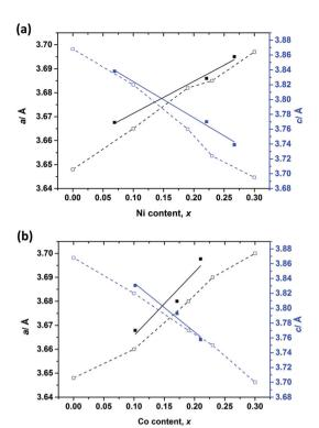
Fig. 4 Variations of unit cell parameters with varying (a) Ni (1-3) and (b) Co (4-6) substitution levels (x). Filled squares show refined values from our PND data. Empty squares show data from ref. 11. Trend lines serve as a guide to the eye.
