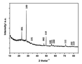
Fig. 2 Typical XRD pattern of a  $\text{Li}_{3-x-y}M_xN$  sample (M = Co-Cu) synthesised by MW methods (sample 2 is shown). Indices for the expected reflections are indicated.
