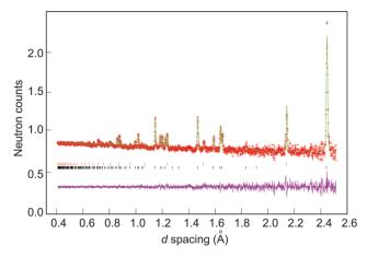
Fig. 3 Rietveld fit against PND data collected at room temperature from sample 4 from the  $2\theta=145^\circ$  (backscattering) detector bank. Observed data points are shown in red, calculated profile in green and the difference (obs-calc) profile in pink. Black and red vertical tick marks indicate reflections from the  $\text{Li}_{3-x-y}\text{Co}_x\text{N}$  phase and the vanadium sample can respectively.
