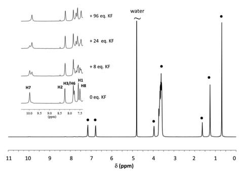
Fig. 3 <sup>1</sup>H NMR spectrum of a 1.5 mM solution of Receptor 2 in 50 mM Triton X-100. Receptor signals are amplified and shown for different additions of KF. ( ) Surfactant signals. The assignment of the receptor signals was made by comparison with the spectrum of the receptor in CTAX micelles. For proton labelling see Fig. 1.
