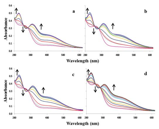
Fig. 2 UV-visible absorption spectra of 2.7 x 10<sup>-5</sup> M 2 in 9:1 DMSO-H<sub>2</sub>O upon addition of various anions as sodium salts: (a) OH<sup>-</sup> (0-4 equivalents), (b)  $F^-$  (0-4 equivalents), (c) AcO $^-$  (0-4 equivalents) and (d)  $H_2PO_4^-$  (0-55 equivalents.).
