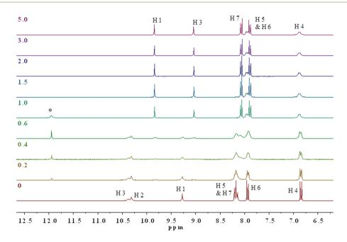
Fig. 5 Stacked  $^{1}$ H NMR spectra of 0.01 M 4 upon addition of AcO $^{-}$  in DMSO- $d_{6}$ -0.5% water at 298 K. Numbers on the left correspond to the equivalence of anions added. The assignments of the  $^{1}$ H resonances are shown for the receptor before and after the addition of increasing amount of TBAAcO. The asterisk \* marks the resonance due to protonation of acetate.
