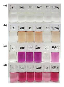
Fig. 1 Colour changes observed for  $2.7 \times 10^{-5}$  M 1–4 in 9:1 DMSO– $H_2O$  on addition of up to 4 equivalents of OH<sup>-</sup>, F<sup>-</sup>, AcO<sup>-</sup>, Cl<sup>-</sup> and  $H_2PO_4$ <sup>-</sup> as sodium salts.
