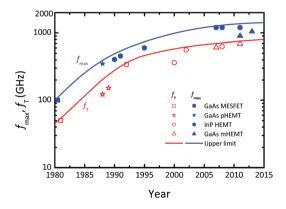
Fig. 3 Evolution of the cutoff frequency  $f_T$  and maximum frequency of oscillation  $f_{\text{max}}$  of RF FETs. Shown are the record  $f_{\text{T}}$  and  $f_{\text{max}}$  values reported at a certain time. MESFET: metal-semiconductor FET; HEMT: high electron mobility transistor; pHEMT: pseudomorphic HEMT; mHEMT: metamorphic HEMT. Data are taken from ref. 20-39.
