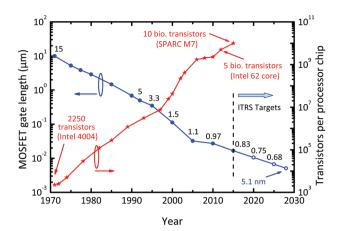
Fig. 2 Evolution of the MOSFET gate length and the number of transistors integrated on a single microprocessor chip. The numbers above the gate length curve indicate the processor supply voltage  $V_{\rm DD}$ . Note the continuous decrease of  $V_{\rm DD}$  in the past and the required continuation of this trend in the future. The ITRS targets refer to MOSFETs for high-performance logic as specified in the 2013 ITRS edition.<sup>7</sup>
