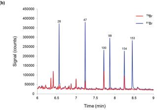
Fig. 5 Chromatograms obtained by GC-ICP-MS for (a) mineral water (blank sample) and (b) a river water sample both spiked with <sup>81</sup>Br-labelled PBDEs.
