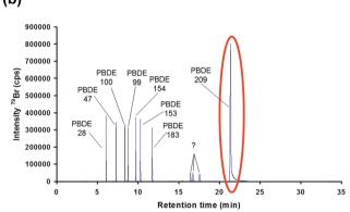
Fig. 3 Effect of the GC capillary position inside the interface placed (a) 0.2 cm before the injector tip exit and (b) 10 cm beyond the Ar carrier gas inlet to the interface inside the GC oven.
