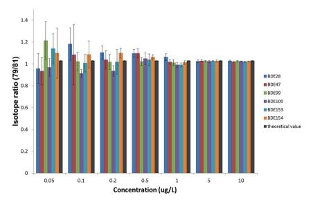
Accuracy and precision of isotope ratio measurements achieved by GC-ICP-MS under the optimized experimental working conditions.
