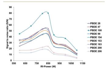
**Fig. 2** Effect of the RF power settings on the signal to noise ratio of the selected PBDE congeners when using GC-ICP-MS conditions. Calculations were based on the <sup>79</sup>Br signal.
