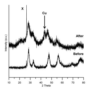
**Fig. 1** pXRD pattern of Cu/HSACeO<sub>2</sub> catalyst before and after reaction. Only one peak can be tentatively assigned to a Cu or CuO phase either before or after reduction. The pattern for the catalyst after reaction indicates a more amorphous structure possibly due to the formation of Ce<sub>2</sub>O<sub>3</sub> phases [The sharp peak at 26  $2\theta^{\circ}$  X is from the brass insert used in the sample holder].
