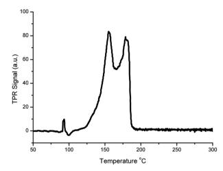
Fig. 2 Results of temperature programmed reduction of the unreduced Cu/HSACeO<sub>2</sub> catalyst immediately following calcination; two well separated peaks can be seen at 155 and 178 °C, these two peaks are tentatively assigned to non-crystalline CuO interacting with CeO<sub>2</sub> and larger non-crystalline CuO associated with CeO<sub>2</sub> respectively.
