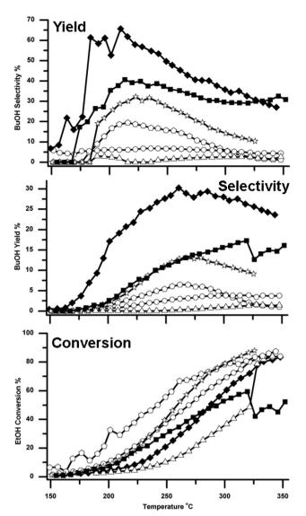
Fig. 3 Traces showing how the yield of BuOH, selectivity to BuOH and conversion of EtOH, vary over the six different catalysts. The traces are marked as follows  $\bigcirc$  Cu/Al<sub>2</sub>O<sub>3</sub>,  $\triangle$  Cu/ZSM-5 SAR-80,  $\updownarrow$  Cu/TiO<sub>2</sub>,  $\bigcirc$  Cu/Si/ Al, ■ Cu/CeO<sub>2</sub> and ◆ Cu/HSA CeO<sub>2</sub>. Note that, although the yields varied, some BuOH was formed over all six catalysts.
