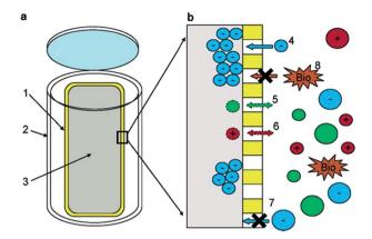
Fig. 2 (a) Schematic showing the components of the passive sampler. (1) Poly(vinylidene fluoride) membrane. (2) High-density polyethylene casing. (3) Diethylaminoethyl-cellulose resin. (b) Region showing the resin/membrane/water interface. (4) Negatively charged DOM enters the membrane and is sorbed onto the resin, (5 + 6) neutral or positively charged DOM is not retained. (7 + 8) Large species cannot enter the membrane. Reproduced with permission from Lam  $et\ al.^{119}$
