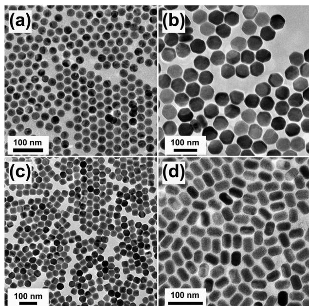
Fig. 5 Low-resolution TEM characterization of lanthanide-doped UC nanocrystals (unpublished results). (a) NaYF<sub>4</sub>:Yb/Er (18/2 mol%) spherical nanocrystals. (b) NaYF<sub>4</sub>:Yb/Tm (49/1 mol%) nanoplates. (c) NaYF<sub>4</sub>:Yb/Tm (20/0.2 mol%)@NaYF<sub>4</sub> nanoprisms. (d) NaYF<sub>4</sub>:Yb/Er (18/2 mol%)@NaYF<sub>4</sub> nanorods. Note that all these nanocrystals were prepared by the co-precipitation method.
