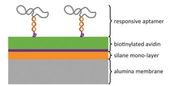
Fig. 1 Modular architecture of the small-molecule stimuli-responsive membrane. The thickness of the support structure comprising the silane and avidin layers may be adapted depending on the size of the responsive receptor molecule (aptamer) and the pore size of the base material (AAO membrane).
