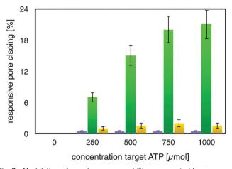
Fig. 2 Modulation of membrane permeability, represented by degree of pore closing, through specific recognition of ATP (green) by the ATPaptamer modified AAO-membrane. Only a minor non-specific responsiveness was observed toward GTP (yellow); the AAO-membrane modified with a mutated ATP-aptamer exhibited a negligible response upon exposure to the ATP-target (violet).
