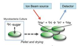
Fig. 1 Schematic illustration for assessing <sup>2</sup>H-carbohydrate uptake by M. smegmatis and ion beam analysis.
