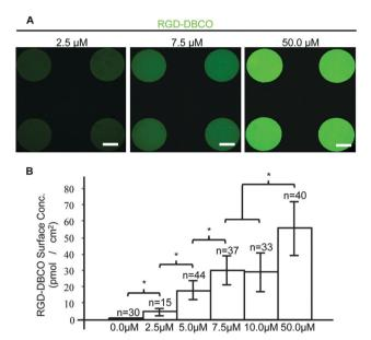
**Fig. 1** (A) Fluorescent images of micropatterned PEGMA brushes conjugated with RGD–DBCO at varying reaction concentrations, 150  $\mu$ m scale bars. (B) Surface density of RGD–DBCO on micropatterned substrates across all reaction concentrations, \*p < 0.05.
